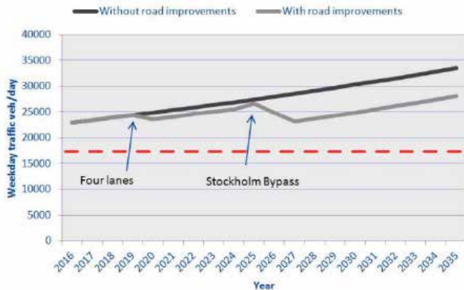
Fig. 5.2: Expected traffic flow on E4 from 2016 - 2035 on Drottningholm Bridge based on available traffic projections. The black line illustrates an annual traffic increase of 2 % if no measures are taken (evaluation). The grey line shows the impact of the road projects, compared to this. The red dashed line shows the traffic rate at the time of the inscription of the World Heritage property (1991, 26 700 cars). It is clearly visible that traffic will increase in phase 1 and phase 2 if no regulation measures are taken (© Swedish Transport Administration).
